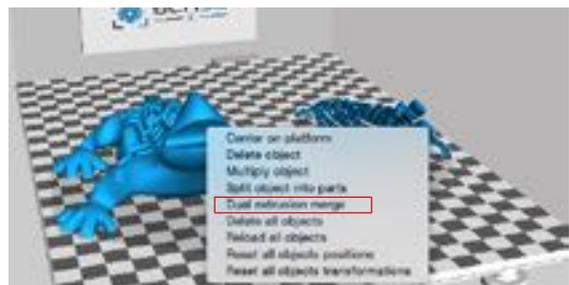
2. Click on File. Load Draudi profile and select the \*.STL format files to be printed. After you have done this, the Draudi object will appear in two parts.
