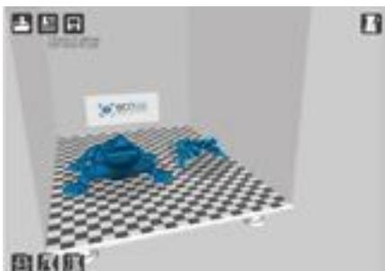
4. The figure should now appear as a single model in two different colours. This process may take a few seconds.
