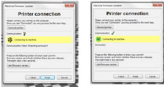
7. After the printer is connected, click on Get Firmware Version. This button compares the printer's version of the firmware with GitHub's latest version, and will display an update option if a new version is available.
